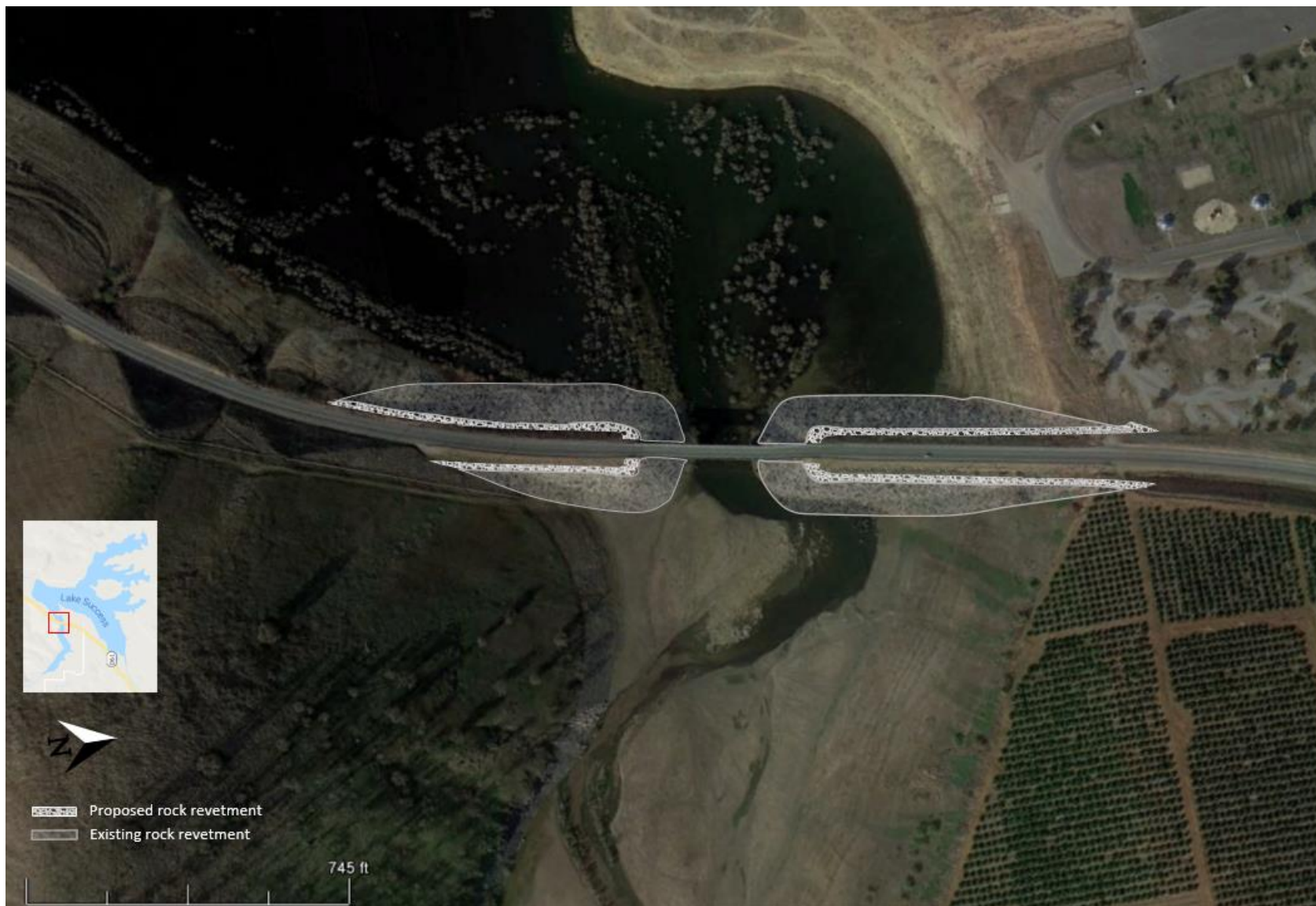
Figure 6. Proposed additional 10 feet of rock revetment placement along the Highway 190 bridge abutments for erosion protection in Phase 2 of the Tule River Spillway Enlargement Project.
